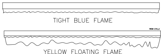
Figure 20 - Main Burner Flame
